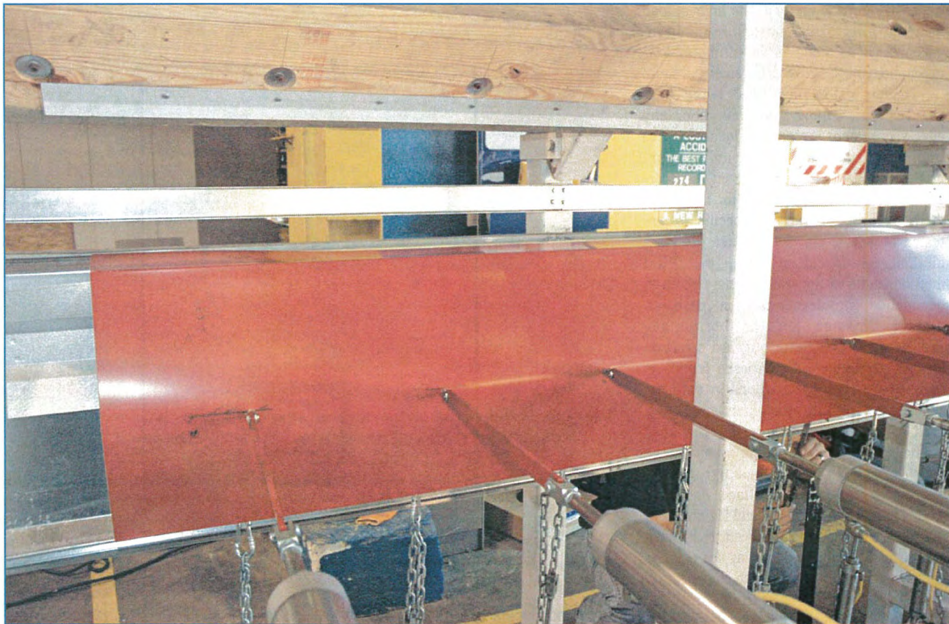
Figure 3 – RE-3 pull-off test for copings. Photo courtesy of Hurricane Test Laboratory and IMETCO.
