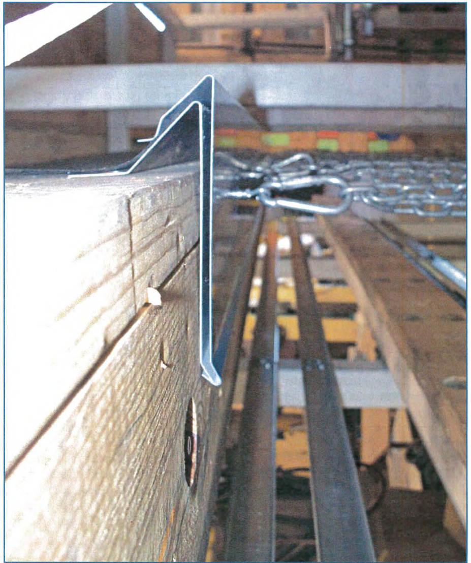
Figure 2 – RE-2 pull-off test for edge flashing. Photo courtesy of Hurricane Test Laboratory and IMETCO.
